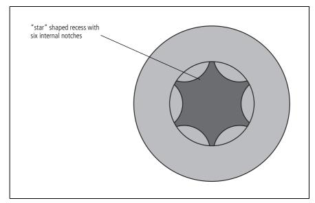
Figure 1.2 Identifying Torx Screws
