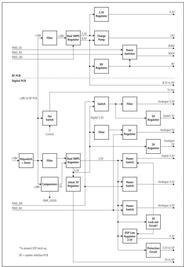
The +3.3V output is distributed to the remaining circuitry and to the +2.5V regulator for the DSP. These are switched as part of the power saving modes. The +3.3V output is also supplied to the system interface PCB via a protection circuit.
