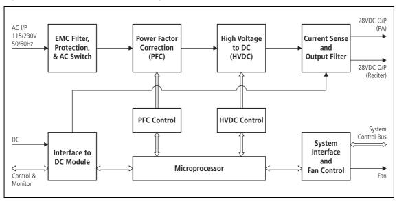
Figure 6.3 PMU AC Module Block Diagram
