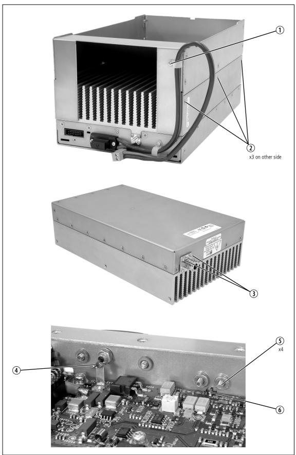
Figure 5.2 Removing the Airflow Duct, Cover and Front Panel
