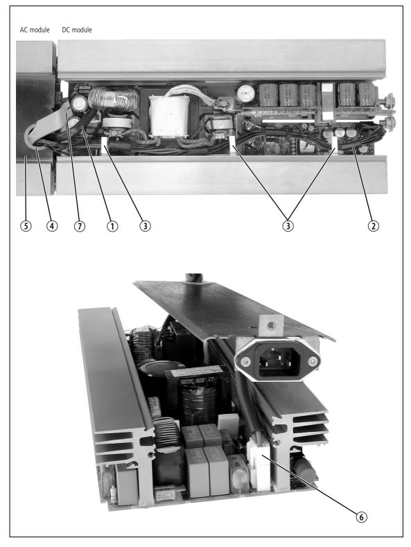
Figure 7.3 Reconnecting the AC and DC Modules
