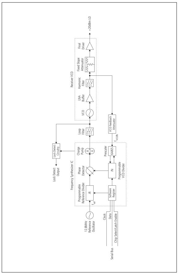
Figure 2.6 Reciter Receiver Synthesizer Block Diagram
