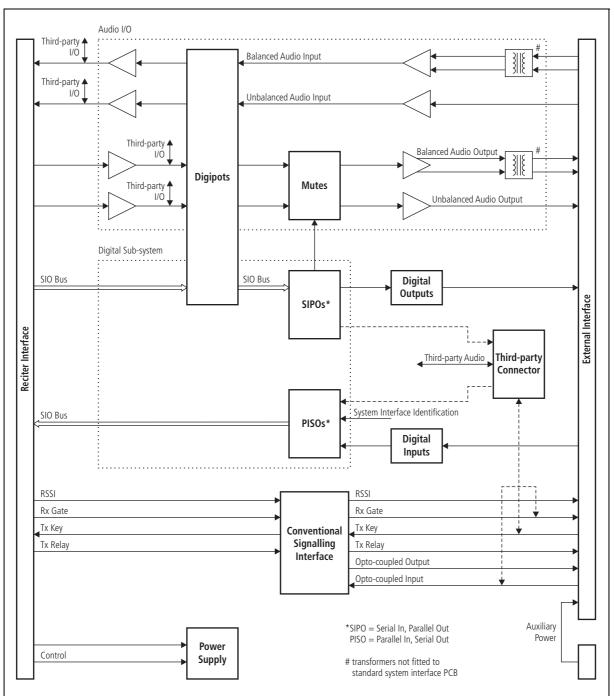
Figure 2.9 Reciter System Interface PCB Block Diagram
