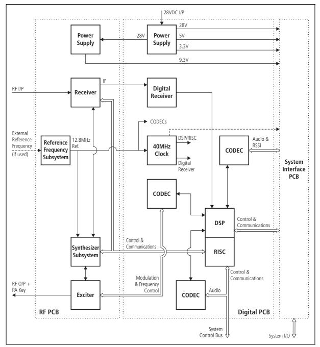
Figure 2.1 Reciter High Level Block Diagram
