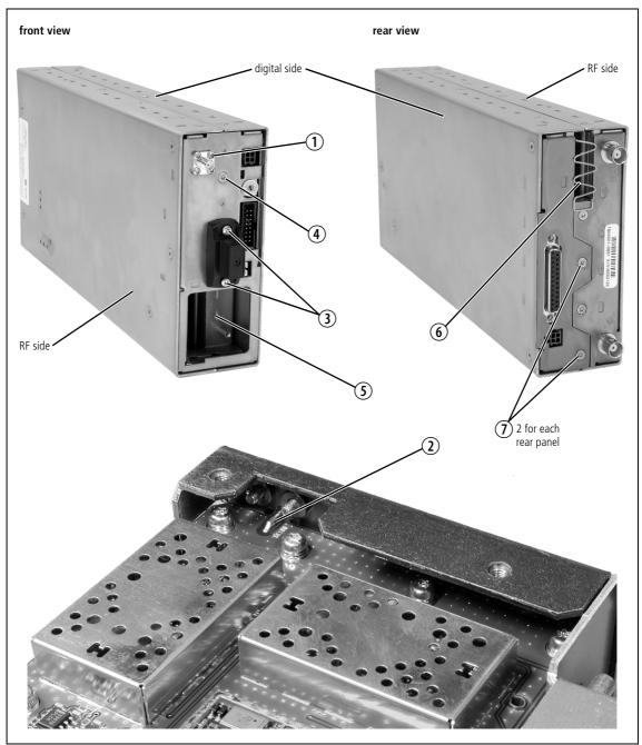
Figure 3.2 Removing the Front and Rear Panels
