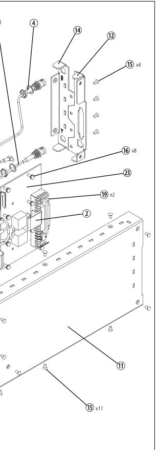
TB8100 Service Manual © Tait Electronics Ltd April 2004 The TB8100 power amplifier (PA) is a modular design with the circuitry divided between separate PCBs. These PCBs are assembled onto a heatsink in different configurations in different models.
