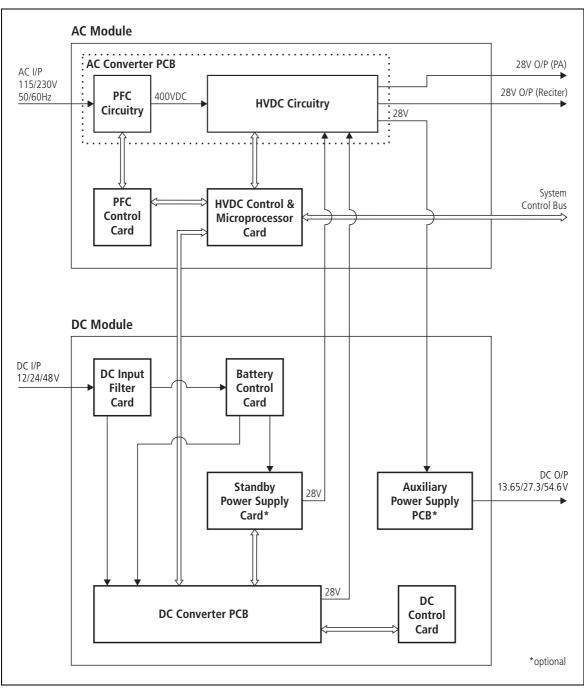
Figure 6.1 PMU High Level Block Diagram
