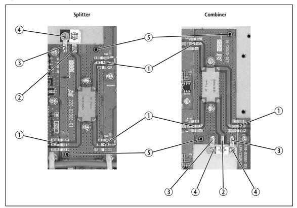
Figure 5.9 Replacing the Splitter/Combiner PCBs
