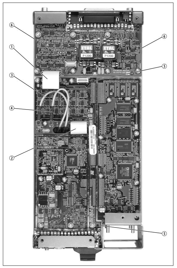
Figure 3.3 Replacing the Digital and System Interface PCBs
