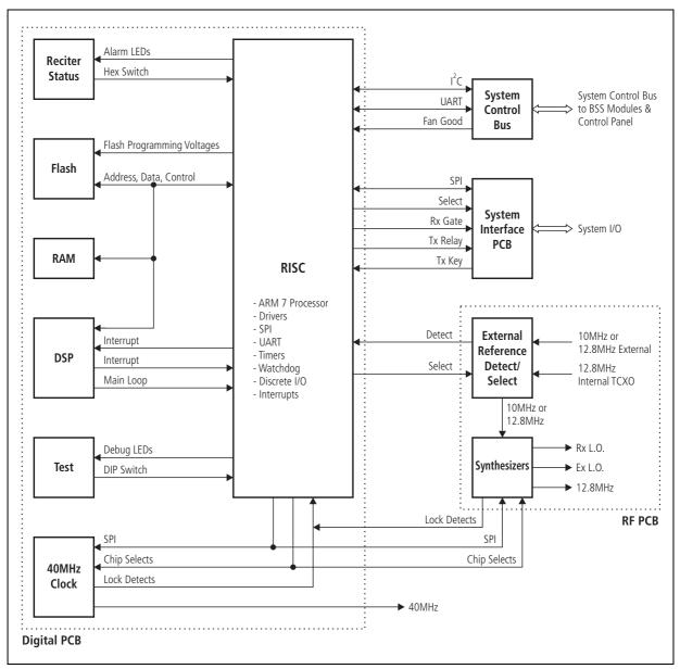
Figure 2.3 Reciter RISC Functional Block Diagram
