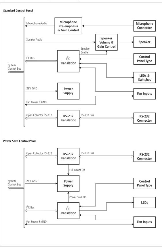
Figure 8.1 Control Panel High Level Block Diagrams
